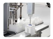
The coverglass is taken by a suction cup electronic system while the dispensing needle moves from its stand-by position in the solvent.
