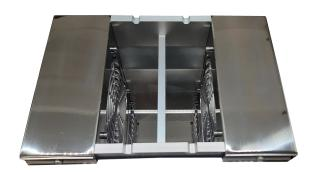
The slide stainer can be equipped with a 2-station drying system, each station is provided with a heater and fan. The two units are operated simultaneously so to keep temperature constant.
