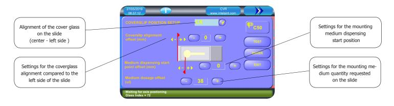
Precise setting of the coverglass on the slide and of mounting medium dispencing are provided thanks to the CVR sofisticated mounting unit.
