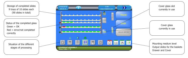
The intuitive operator interface allows the user to always have all the different working stages under control
