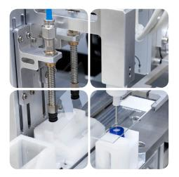
The mounting medium (500 ml bottle), is studied to be easily accessible, with rapid connections (level sensor included) which allows the operator to substitute the bottle without touching any wire.
