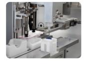
The coverglass is mounted through a particular movement of the suction cup system which avoids bubble air formation
